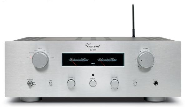
Also the inputs of the amplifier have been changed. Now the new SV-228 has a Bluetooth input (vers. 5.0) for wireless streaming.
